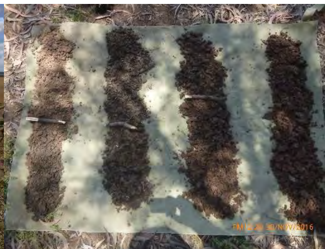
Site APA-16 soil profile, surface at top left, 30 cm sections
