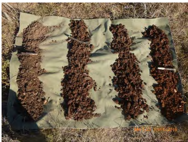
Plate 3-9 Soil profile at site #23, surface top left, 30 cm sections to 1.2 m. acidic Brown Dermosol
