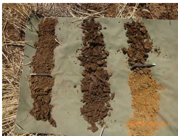
Plate 3-16 Soil profile at site #38, surface top left, 30 cm sections to 0.9 m. Brown Vertosol overlying weathered mudstone at 0.75 cm
