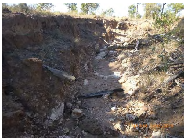
Plate 3-17 Gully erosion at site #24 showing sandstone parent material exposed at its base
