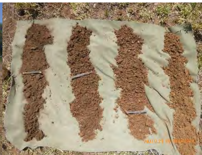
Site APA-14 soil profile, surface at top left, 30 cm sections
