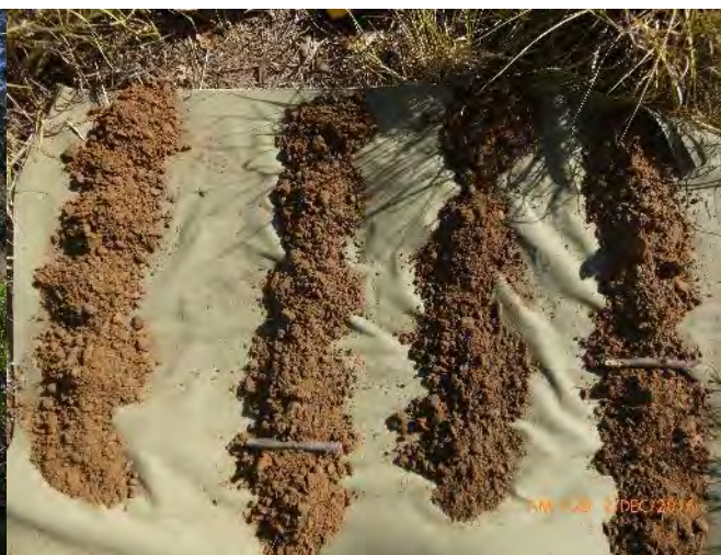
Site APA-35 soil profile, surface at top right, 30 cm sections
