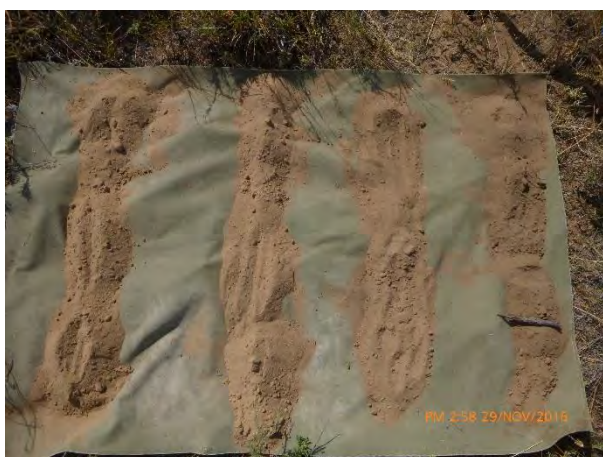
Plate 3-1 Soil profile at site #10 with surface top right in 30 cm sections to 1.2 m, showing deep sandy apedal profile
