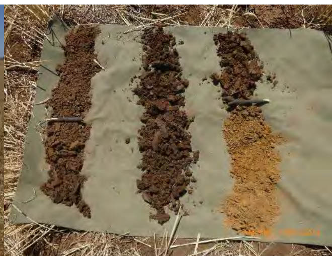
Site APA-38 soil profile, surface at top left, 30 cm sections
