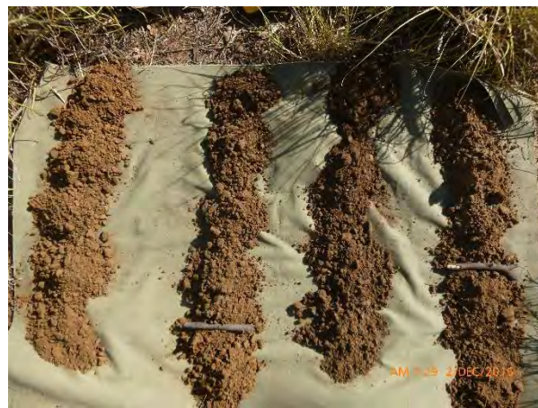
Plate 3-4 Soil profile at site #35 surface top right, 30 cm sections to 1.2 m, showing deep moderate to well-structured Brown Dermosol
