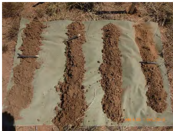
Plate 3-12 Soil profile at site #25, surface top right, 30 cm sections to 1.2 m. Brown Dermosol with weak to moderate structure in the subsoil
