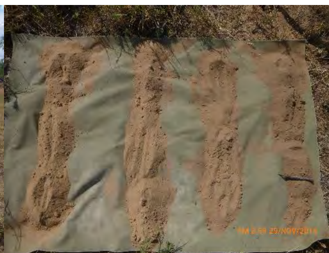
Site APA-10 soil profile, surface at top right, 30 cm sections
