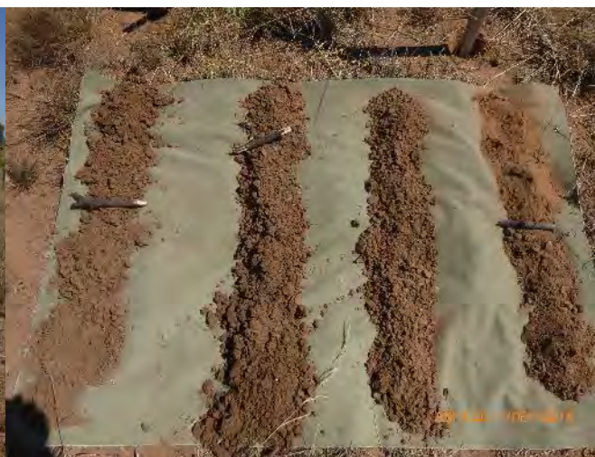
Site APA-25 soil profile, surface at top right, 30 cm sections
