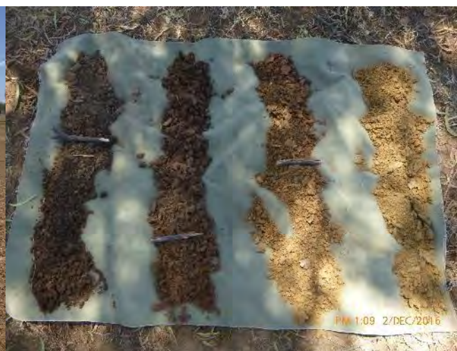
Site APA-42 soil profile, surface at top left, 30 cm sections
