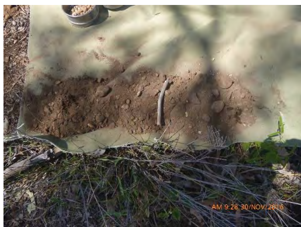
Plate 3-23 Soil profile at site #13, surface left hand side, excavation stopped by weathered sandstone
