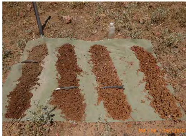
Plate 3-6 Soil profile at site #29, surface top left, 30 cm sections to 1.2 m. Brown Dermosol
