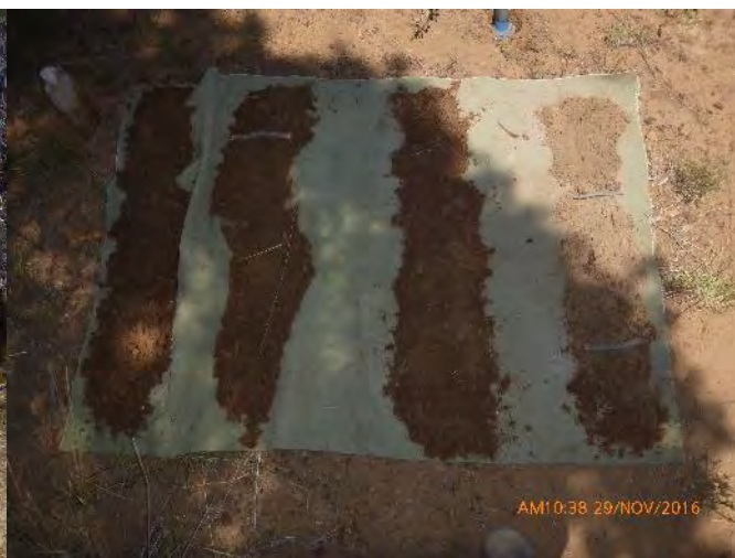
Site APA-4 soil profile, surface at top right, 30 cm sections
