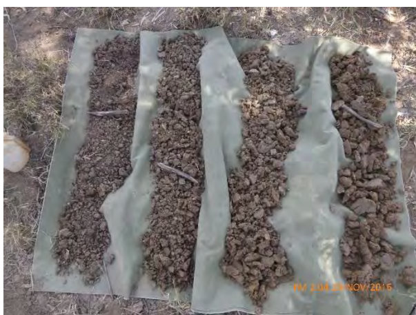
Plate 3-15 Soil profile at site #8, surface top left, 30 cm sections to 1.2 m. Brown Vertosol with grey surface
