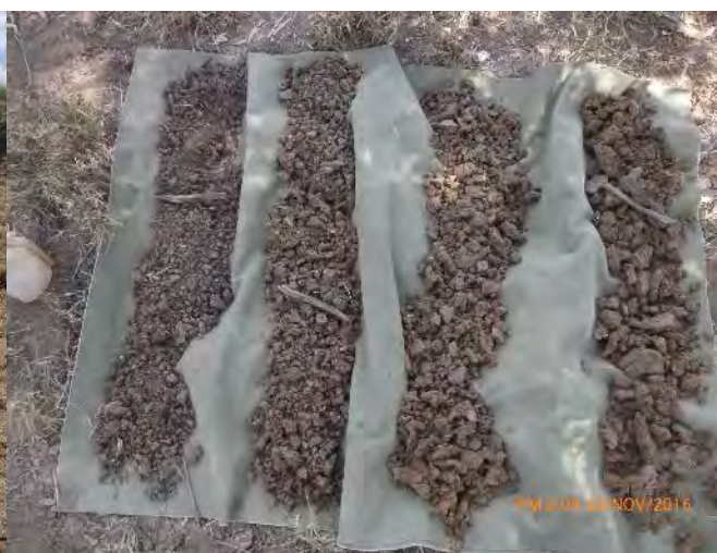
Site APA-8 soil profile, surface at top left, 30 cm sections
