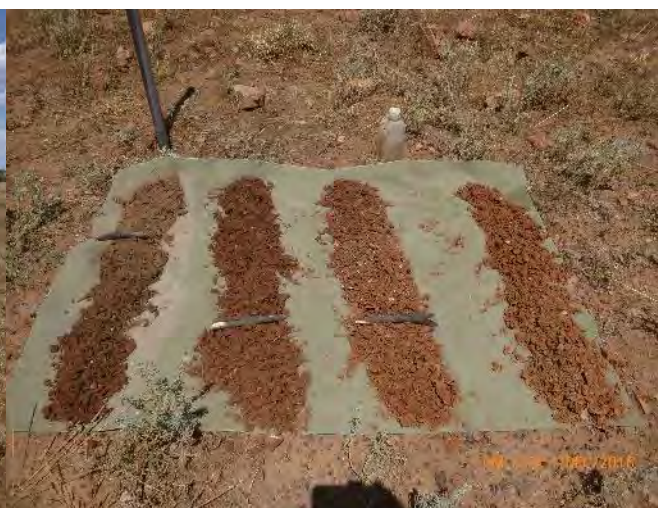
Site APA-29 soil profile, surface at top left, 30 cm sections
