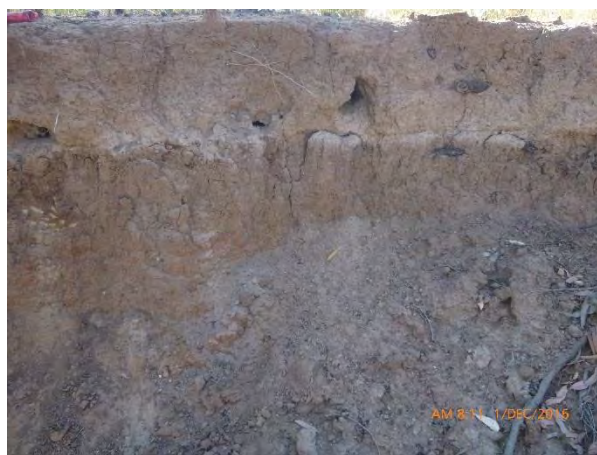
Plate 3-18 Soil profile at site #24 with sandy clay loam surface over columnar structured subsoil
