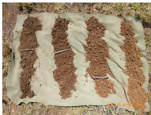
Plate 3-8 Soil profile at site #14, surface top left, 30 cm sections to 1.2 m. alkaline Brown Dermosol
