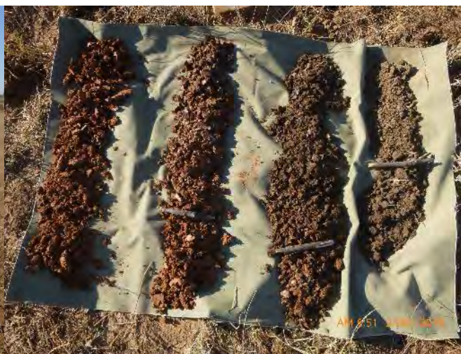
Site APA-34 soil profile, surface at top right, 30 cm sections
