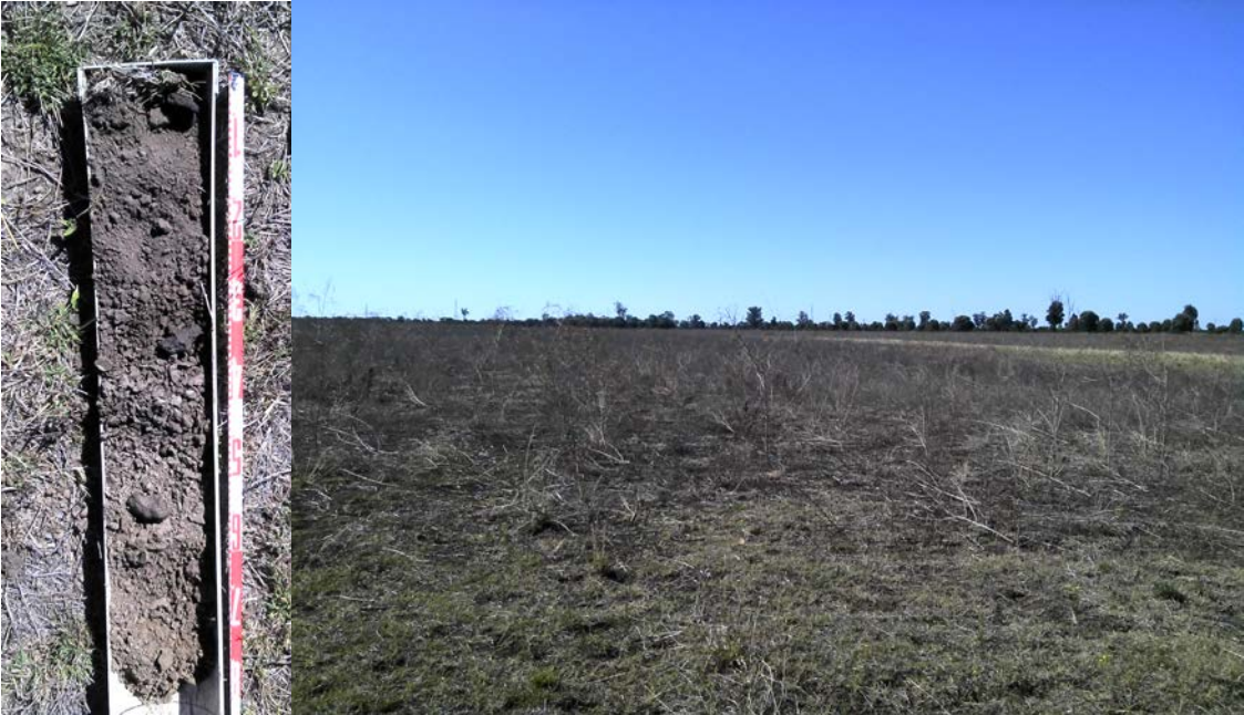
Figure 2: Soil profile for Site 1: Moderately self-mulching cracking Clay
