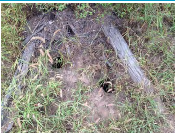
Site S1 surface condition, tunnel erosion
