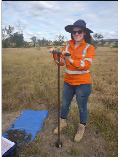
Photo 1 Hand auger used for representative soil profile and shallow subsurface observations
