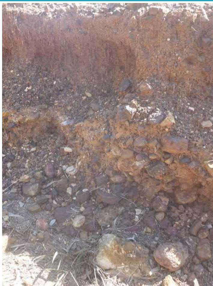
Site W02 watercourse bank profile, severe bank erosion, precipitous (>100%) bank approx. 1.5 m high
